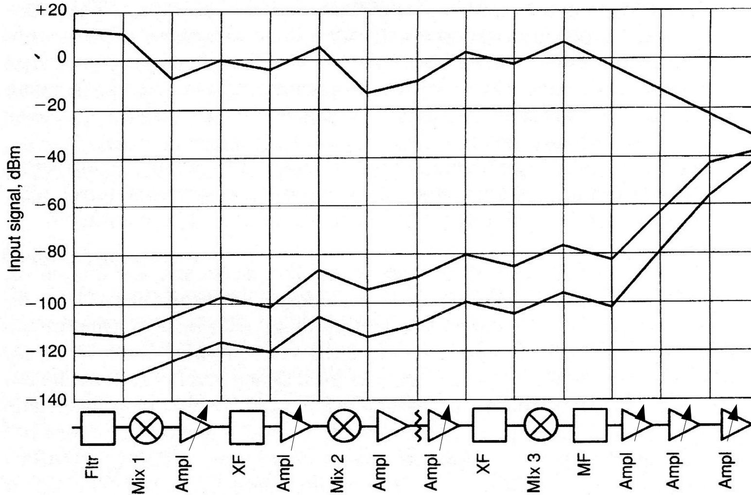
**Figure 4.28** The power level for three conditions of signal input is plotted for each stage to plan the gain and AGC distribution.
